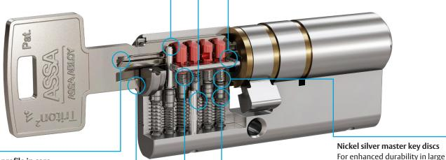
Paracentric profile in core Provides resistance to pick attack
